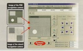
Print inspection camera High-speed capture is executed by the digital camera with high resolution and wide field-of-view.
