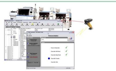
SMS Linecheck confirms that the new reel is the correct part and is the same part as the exhausted reel
